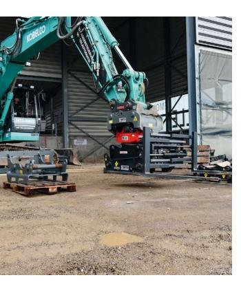
KAUP Fork Positioners are an important accessory of the construction machine, especially when the widths of the loads change constantly. Adjustment of the distance between forks accommodating to different
