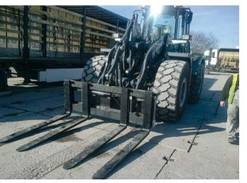
KAUP Sideshifters allow lateral shift of the load, taking the capacity of the construction machine into account, of  $\pm$
