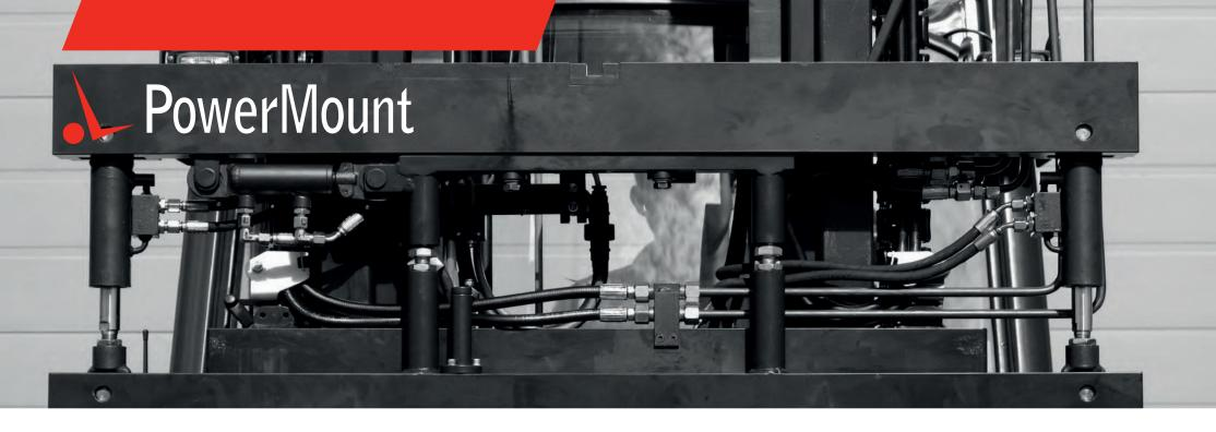
PowerMount, from B&B Attachments is a quick release system which provides a faster, easier and safer way to interchange forklift attachments. Attachments can now be safely engaged and disengaged by the driver in 60 - 90 seconds, making your forklift fleet highly flexible and more cost effective.
