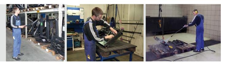
All wear and tear parts are carefully checked and, if necessary, replaced. The fork thickness is checked with regard to the permissible nominal thickness and built up or replaced as necessary. After re-painting the attachment is re-assembled and intensively tested on the test stand. The result of our premium quality standard ensures that you receive a technically flawless used attachment which is as good as new which can be put into operation immediately.
