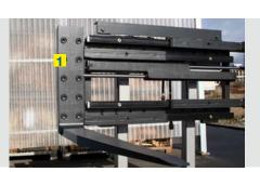
Forks tapered fork width of the carrying part and tapered fork tips
