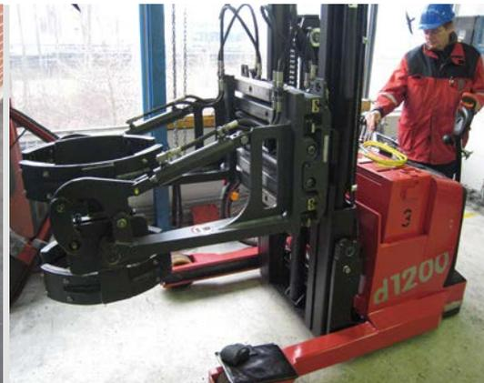
**Drum Clamp T415 · Rotating Drum Clamp T455**
