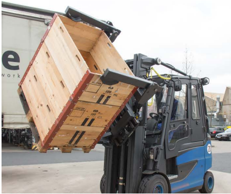
Perfect for emptying boxes based on Euro pallets with a pallet frame.
