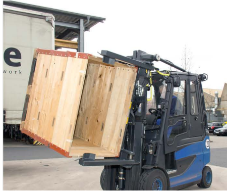
Perfect for emptying boxes based on Euro pallets with a pallet frame.
