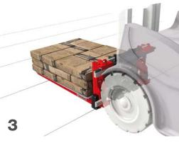
Approach the load, insert the fork tips underneath the load / slip-sheet and activate the conveyer belts.
