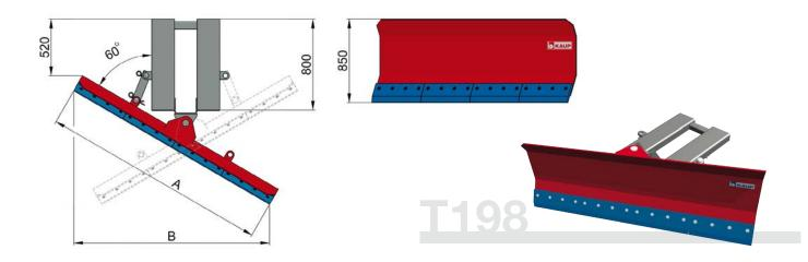
**Snow Plough Blade T198G1/T198FG1**mechanically tiltable - to clear to right or left side - with fork pockets for slipping on forks with a maximum fork cross cut of 160 x 60 mm - distance between fork pockets measured over the outer edges 560 mm
